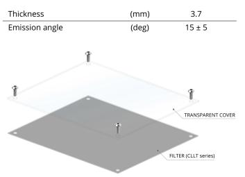
Additional protective window, togheter with its fixing screws, is supplied with the filter
